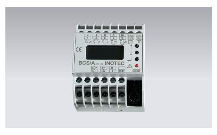
INOTEC Battery-Control-System for monitoring and logging block voltage and temperature of each battery block. Allows early detection and reporting of defective battery blocks. Automatic shutdown of the load and interruption of duration tests due to block failures to protect against destruction of the entire battery.
