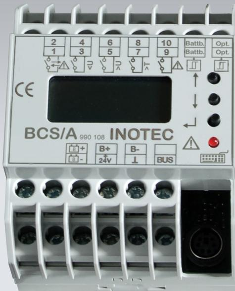
INOTEC Battery-Control-System for monitoring and logging block voltage and temperature of each battery block. Allows early detection and reporting of defective battery blocks. Automatic shutdown of the load and interruption of duration tests due to block failures to protect against destruction of the entire battery.
