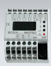
INOTEC Battery-Control-System for monitoring and logging block voltage and temperature of each battery block. Allows early detection and reporting of defective battery blocks. Automatic shutdown of the load and interruption of duration tests due to block failures to protect against destruction of the entire battery.
