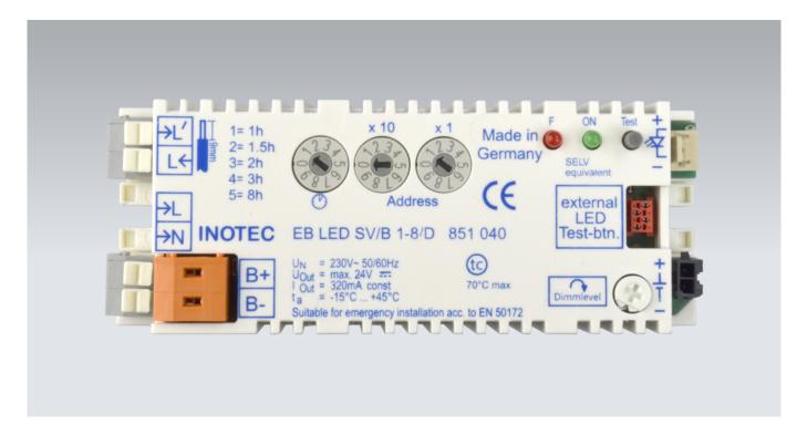
LED-driver with integrated individual lamp monitoring for non-maintained, maintained and switched-maintained lighting. With integrated charging technology and freely selectable nominal operating time of 1h, 1,5h, 2h, 3h or 8h with INOTEC SV/B- function control to connect to a central monitoring device BNS-MTB according to DIN EN 50172, DIN VDE 0100-718 and DIN VDE V 0108-100-1.
