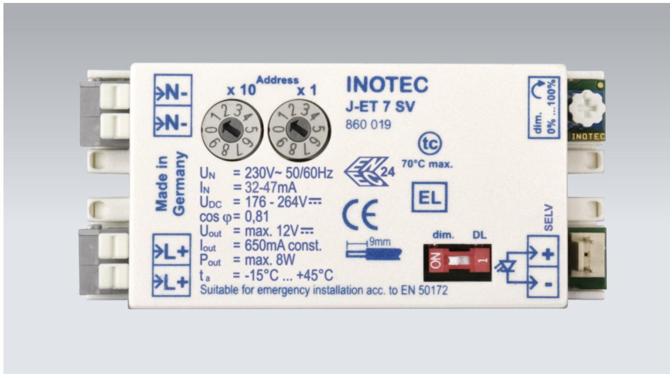
LED-driver with integrated individual lamp monitoring for stand-by and continuous lighting without separate BUS-line. Complying with international standards for safety and working, electromagnetic compatibility and interference resistance. LED output dimmable continuously in mains operation. For connection to JOKER-central battery systems.
