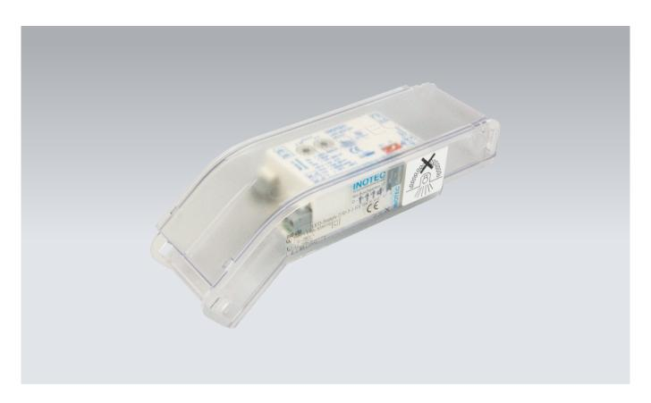
LED-driver with integrated individual lamp monitoring for stand-by and continuous lighting without seperate BUS-line. Complying with international standards for safety and working, electromagnetic compatibility and interference resistance. LED output dimmable continuously in mains operation. For connection to JOKER-central battery systems.
