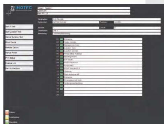
**It is also possible to monitor complex installations containing a range of system types from a single centralised location (using the INOWEB Control software). To perform this process, the CLS 24/SV must be connected to the available network.**
