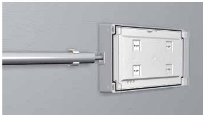
With on-wall installations, pre-moulded lateral openings can simply be punched out. A cable inlet ensures the power cable is inserted cleanly. The separate terminal compartment inside the luminaire further guarantees the high protection rating IP65. There are two mouldings on each of three sides of the luminaire, so that through-wiring is also possible.
