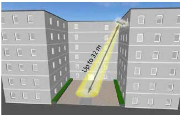
It's often difficult to realise safety lighting at outdoor areas, like it is mentioned in the EN 1838. The supply of luminaires of the general lighting or special mast luminaires are causing high loads. This leads to bigger central power supply units, bigger battery capacities and higher costs.
