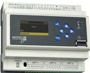
Fully automatic micro-processor controlled monitoring and testing facility to monitor INOTEC emergency network systems with ethernet- and USB-interface. For the inclusion of 3 BUS-monitoring cards with up to 99 addresses each.
