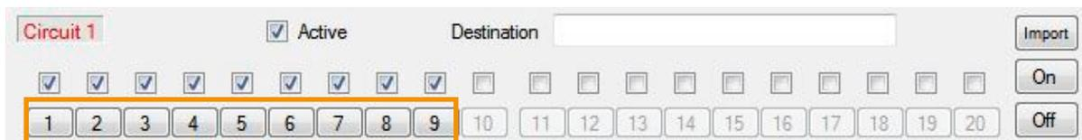
The confirmation of the button with the logical luminaire addresses opens up the dialogue luminaire configuration, in which the settings for the luminaires can be done.
