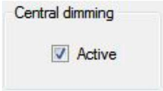
Dimming centrally activates the possibility to dim the luminaires in the final circuit via the CLS dim module. By setting this check box the dim module gets inserted in the switching process.
