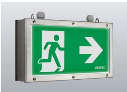
Double-sided emergency exit luminaires made of robust, brushed stainless steel with high protection category. Homogeneous illumination by state-of-the-art LED technology with a luminance of >500cd/m<sup>2</sup>. Suitable for use in food industry or food processing plants with high demands on product hygiene.
