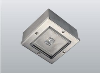
Robust LED safety luminaire with optimised light distribution for the illumination of escape routes with high mounting heights. Also suitable for illumination of firefighting and fire alarm systems as well as first aid stations with 5 lx vertical illuminance. Brushed stainless steel luminaire with high degree of protection. Suitable for use in food industry or food processing plants with high demands on product hygiene.
