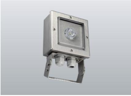
Robust LED safety luminaire with optimised light distribution for the illumination of areas with high mounting heights up to 24m. Brushed stainless steel luminaire with high degree of protection. Suitable for use in food industry or food processing plants with high demands on product hygiene. Lockable mounting bracket to align to the area to be illuminated.
